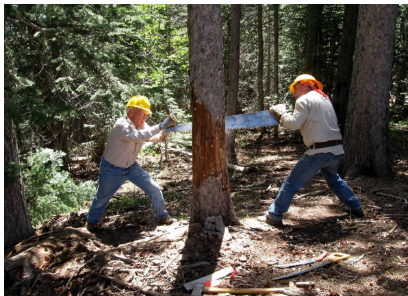
Don Carnicom (L) and Bill White making a sloping face cut in a danger tree with a crosscut saw. Photo by Carl Smith
