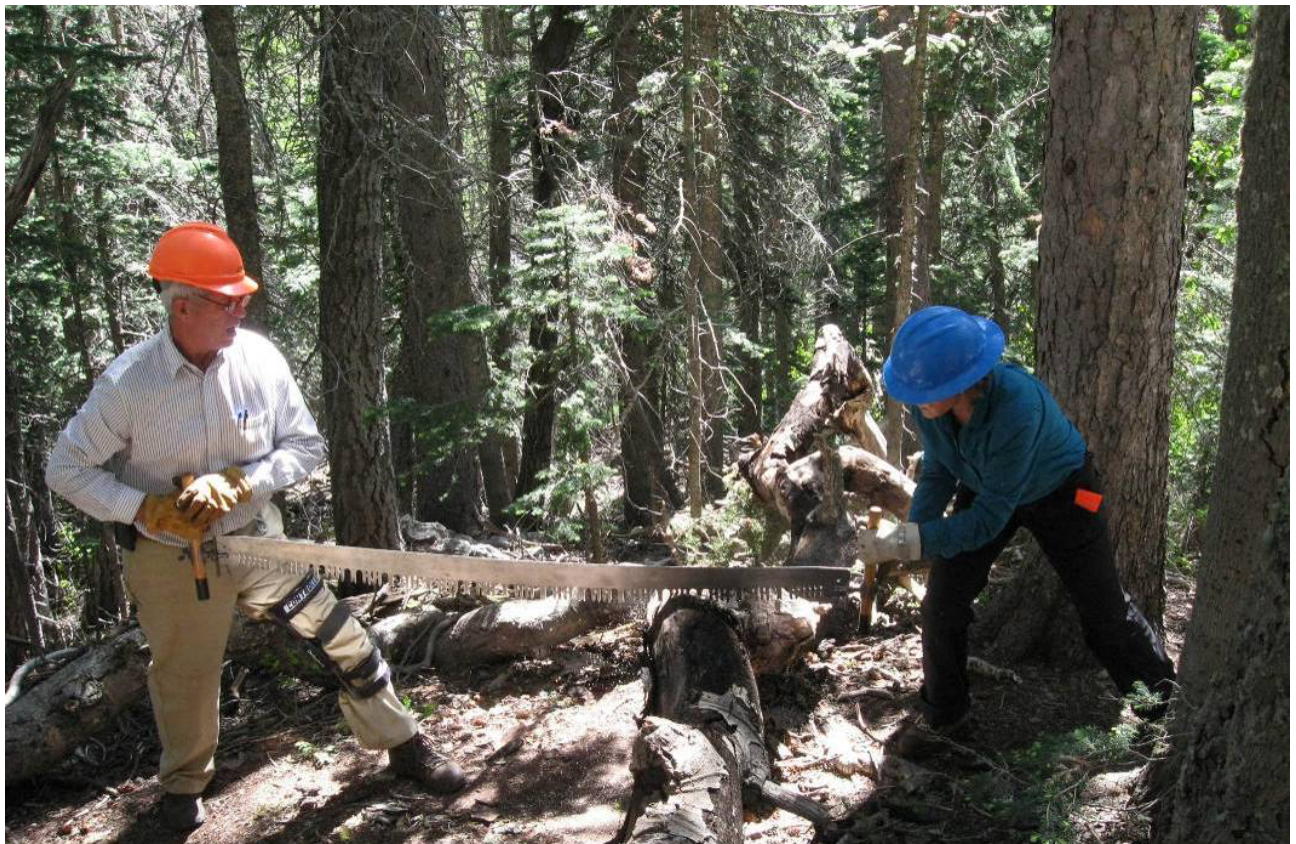
Jim Lunn (L) and Bet Gendron cutting a log with a crosscut saw with perforated lance teeth. Photo by Carl Smith
