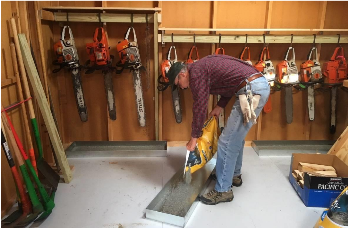
Bob Lowder pouring kitty litter in a steel tray that will go under the chain saws to catch oil drips. (Photo by Sally Lowder)
