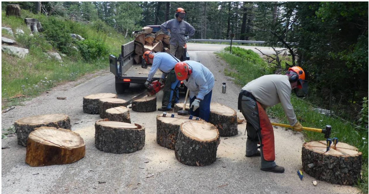
L to R: Dennis Crowther is scoring the Dan's Loop hazard tree rounds with a chain saw to make starting the splitting wedges easier. Joe Meade is standing in his trailer waiting for more wood to stack. Lou Romero and Jim Levesque are splitting rounds. Photo by Sam Beard
