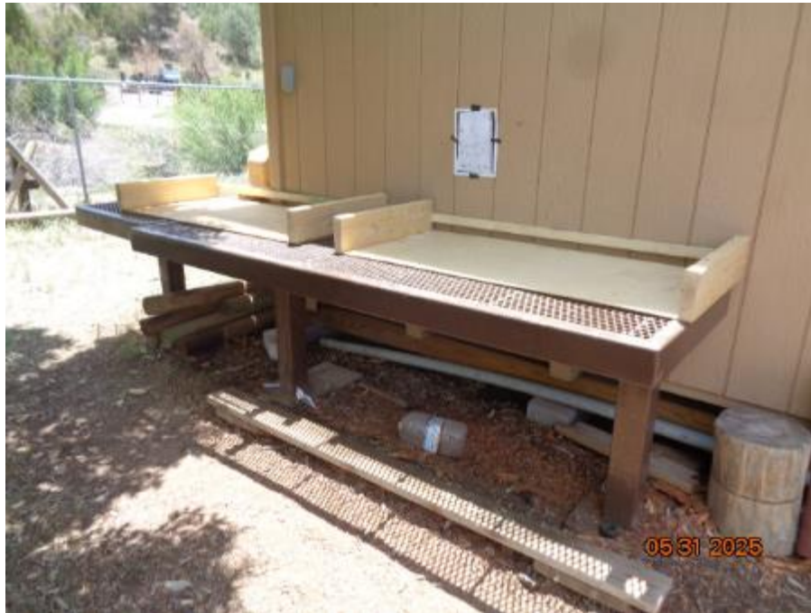
Jigs by Joelle Hertel for making bucks for the buck and rail fence at Kiwanis Meadow. This work area is located at the east end of the FOSM guard station. All photos by Sam Beard
