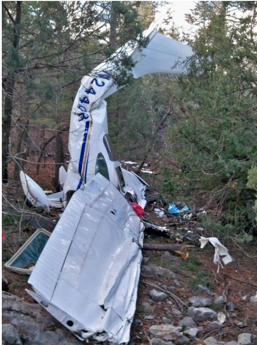
**Cabin and Left Wing. Cabin top cut out to remove bodies. Note dent in front edge of wing at tree.**
