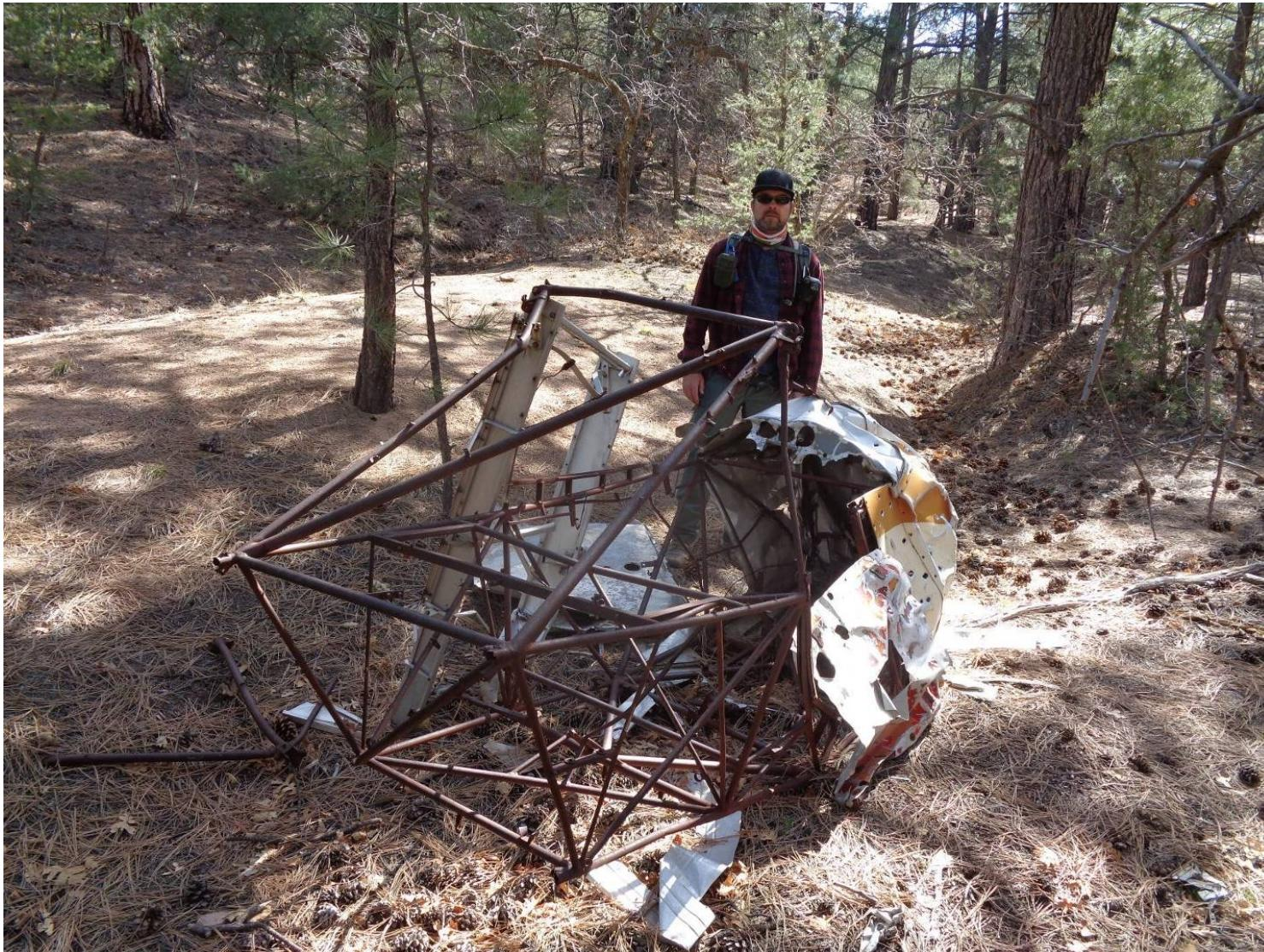
The frame is welded steel tubes.
